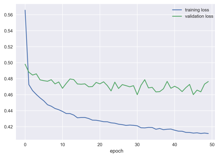
Figure 5. The training loss curve. The blue line corresponds to the training loss. It decreases over epochs indicating the model is learning features from data. The green line corresponds to the validation loss. It first decreases and then becomes relatively steady, meaning the model has converged.
